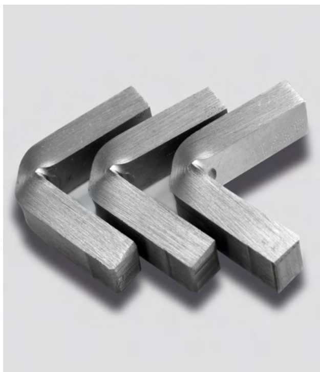
Impact bending samples (tempered to 44 - 46 HRC) after testing on a 450J pendulum impact testing machine
